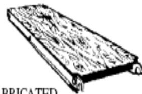
FABRICATED SCAFFOLD DECK
